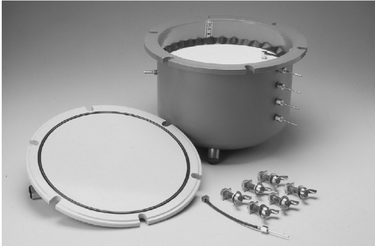
A 5-bar ceramic plate extractor (i.e., maximum applied matrix suction is 500 kPa). (Courtesy of SoilMoisture Equipment Corporation, Santa Barbara, CA).
